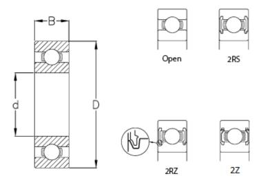
B = 12 Ball grade = 3 C (KN) = 9.95 C0 = 4.75 d = 17 D = 40 Max rpm. = 28000 Type = 6203
